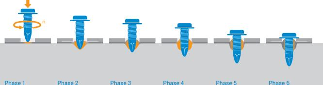
Pressing force and Conical screw tip high RPM heat the penetrates the sheet
