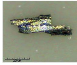
Metal particle from screw thread
