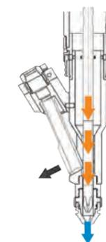
The driving bit advances towards the screw and moves the swivel arm aside so that the following, "on-deck" screw can be fed.
