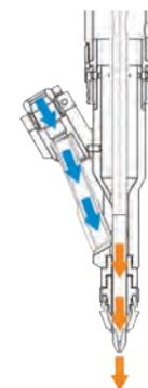
As the screwdriver installs the first fastener, the "on-deck" screw is delivered to the swivel arm. This saves time.
